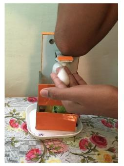
The aluminium strip is affixed with a hinge into a suitable holder, made of scrap plywood and laminate. It may be wall-mounted. Provision of wall fixing is made.
